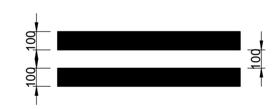
BB - DIVIDING BARRIER LINES (TWO WAY)
