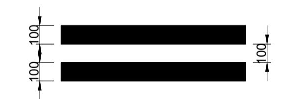
BB - DIVIDING BARRIER LINES (TWO WAY)
