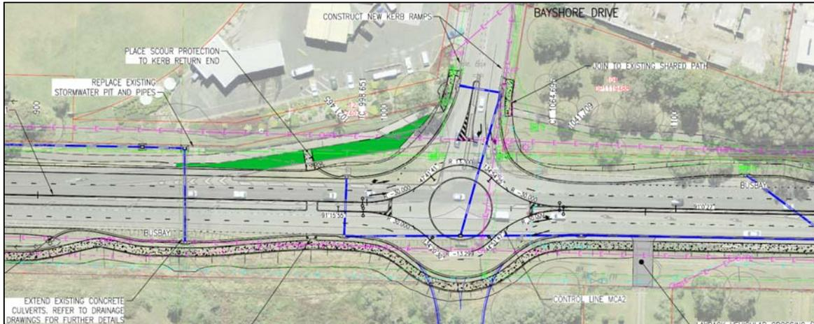
The merge lane length for the upgraded roundabout on Ewingsdale Road with the access to the sports fields indicates a lane and merge length of 202m. To determine the appropriate length to transition from two circulating lanes to one lane reference is made to Austroads Guide to Road Design Part 4B: Roundabouts Clause 4.3.4.
