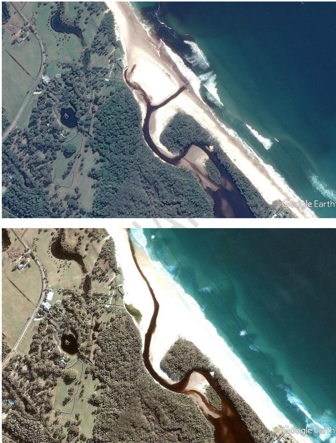
Figure 18 Comparison of Entrance Configuration on 16 May 2013 (Top) and 22 July 2013 (Bottom). The entrance was opened on 13 th May. (Source: Google Earth). Note the tendency towards northwards migration of the entrance channel driven by the dominant south to north alongshore drift.
