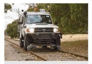
Figure 12: Maintenance Hi-Rail Road/Rail Vehicle
