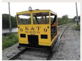
Maintenance speeders: (Source railspeeders.com)
