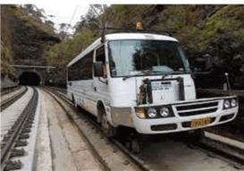
Figure 13: Hi-Rail Bus (22-seater) Wheelchair Access, (Source: TRAINU)
