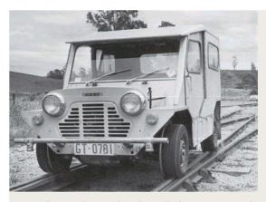
Railway Mokes, used traditionally for transport and maintenance (Source: moke.com.au)
