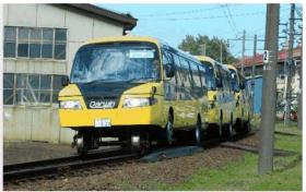
Linked vehicles can fit up to 84 passengers (Source: Asahi.com) Figure 15: DMV Vehicles
