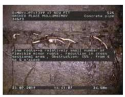
Figure 425 | Root intrusion, Chg 24.50m
