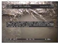
Figure 406 | Root intrusion, Chg 0.00m
