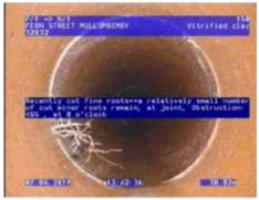
Figure 209 | Root intrusion, Chg 30.82m
