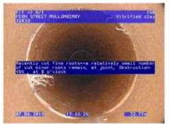
Figure 210 | Root intrusion, Chg 32.77m
