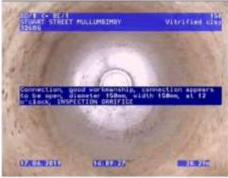
Figure 446 | Inspection point, Chg 20.29m
