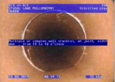
Figure 319 | Cracking, Chg 25.94m
