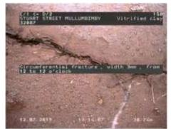
Figure 535 | Displacement, Chg 30.10m
