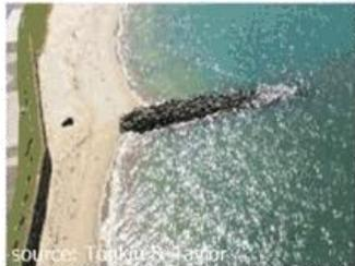
Connect beach in front of revetment and increase sand bypassing on upper beach through construction of a shore-detached groyne. Maintain seaward footprint of existing groyne.
