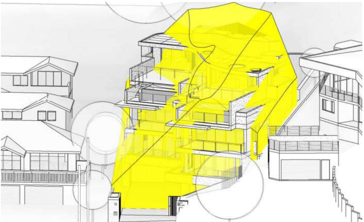
Figure 9 - Building height plane encroachments on southern boundary (non compliant areas are unshaded)
