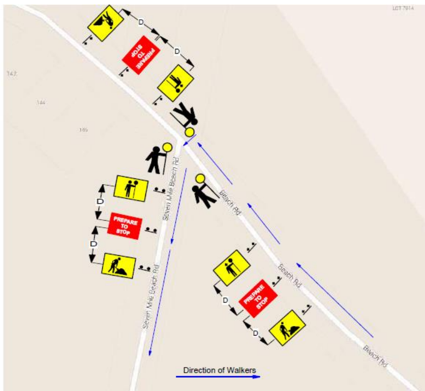
Figure 3 – Proposed TCP for the Seven Mile Beach Rd entrance (refer Figure 2). The Traffic Control is to be in place from 6.30am to 2.30pm.
