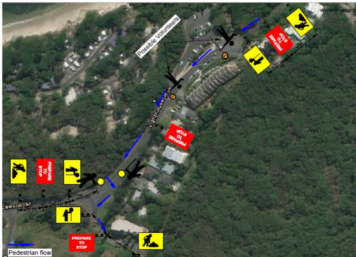
Figure 5 – Traffic control proposed for the western section of Lighthouse Road entering Tallows Beach Road (refer to Figure 2). Traffic control to be in place between 6am to 12.30pm.
