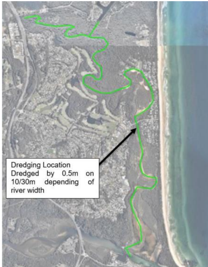
Diagram 32: Option MC – Marshalls Creek Dredging (page 109 of the Flood Study)
