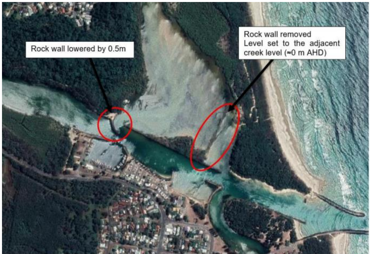
Diagram 28: Option RW – Rock wall modifications (page 103 of the Flood Study)
