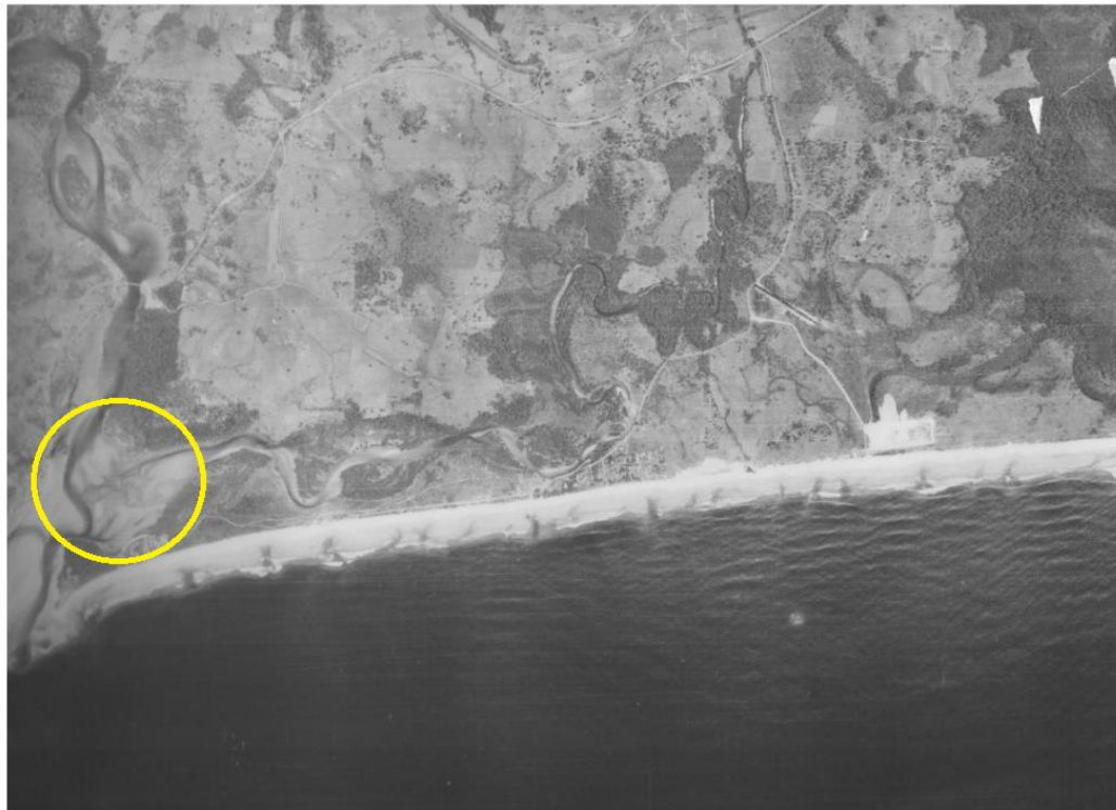
Aerial Photo (dated 1958) flood_story33 (brunswickvalley.com.au) with with yellow circle outlining sandy flood tide delta pre-construction of river walls.
