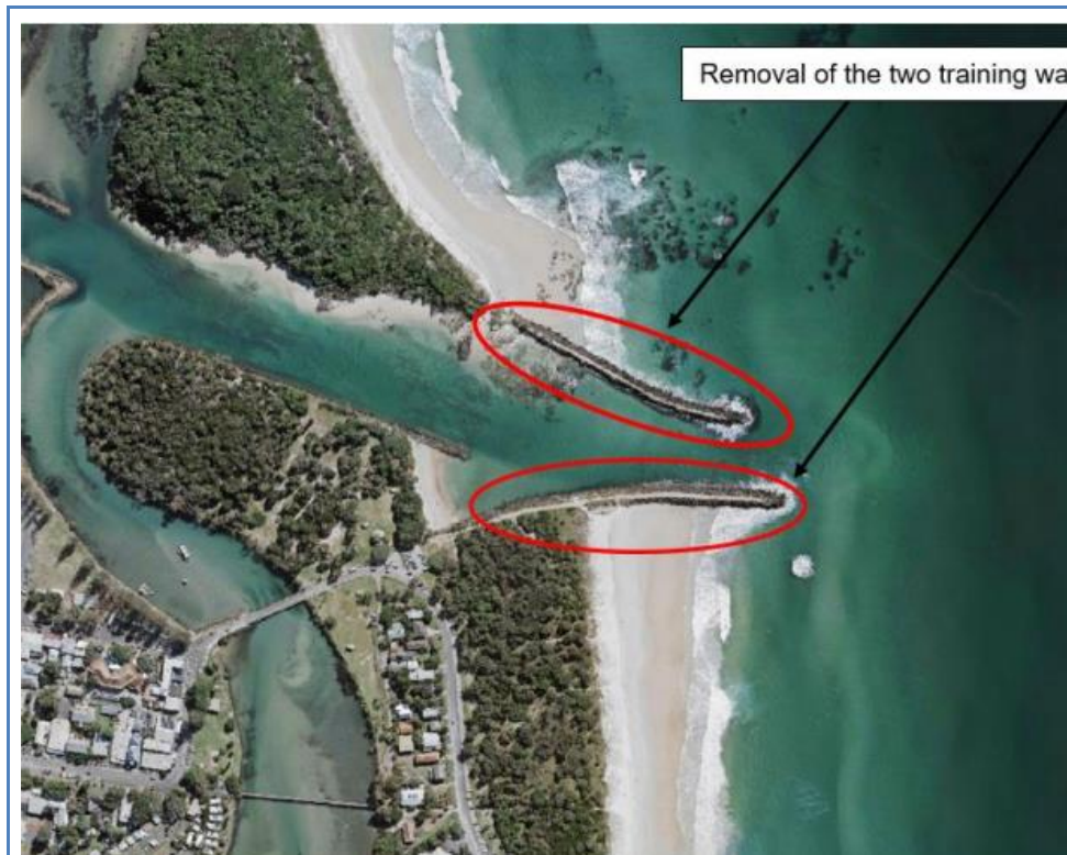
Diagram 29: Option TW – removal of Brunswick River training walls (page 104 of the Flood Study)
