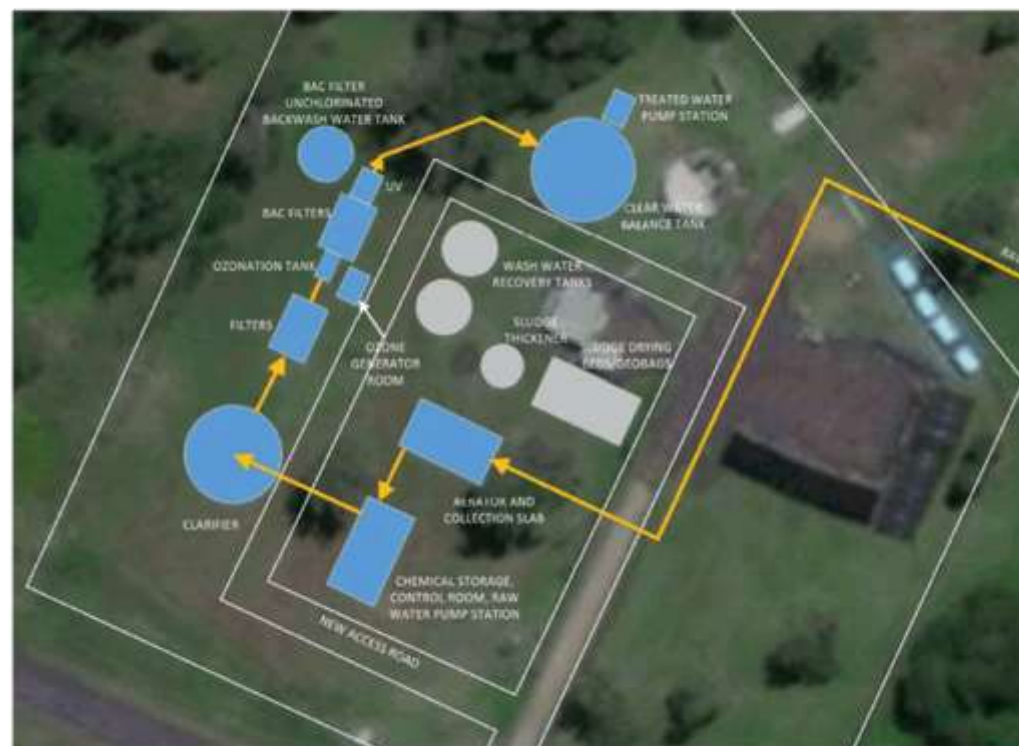
Figure 4.3 : Concept Layout for new Groundwater Treatment Plant
