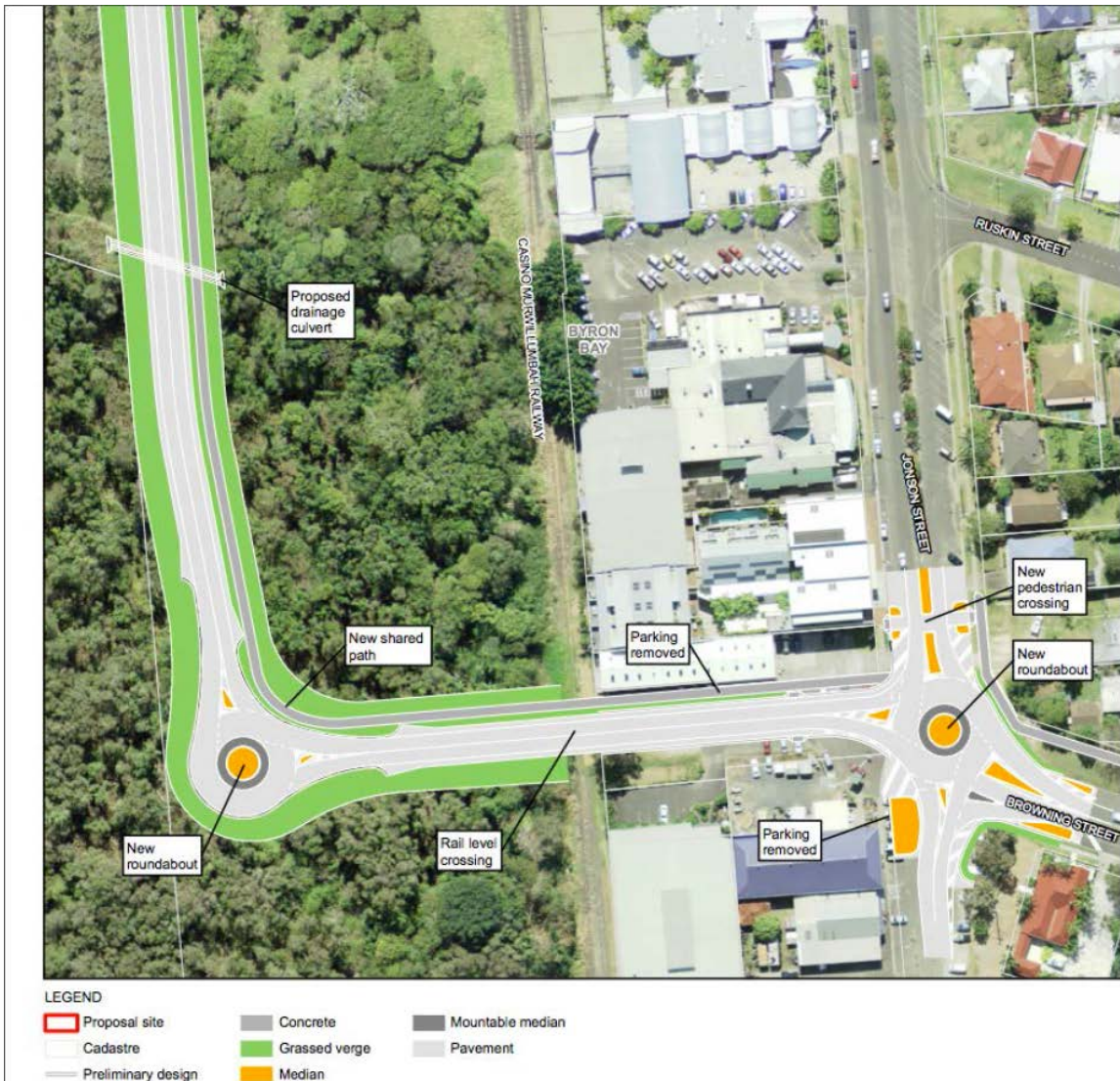
Figure 8 - The Byron Bay Bypass provides a 2.5m shared path separated from the roadway for the full length of the project.
