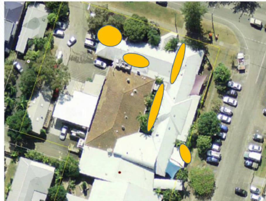
Figure 1 - 10-12 Shirley Street – areas of elevated radioactivity (above background levels) highlighted in yellow
