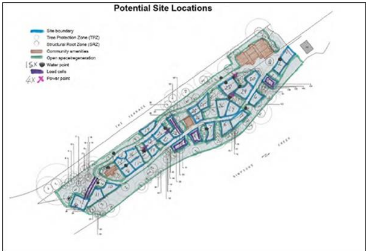
Fig 1: Proposed site plan from the Arboricultural Report showing potential site locations, regeneration/open areas, load cell installation sites, water and power points, and tree positions.
