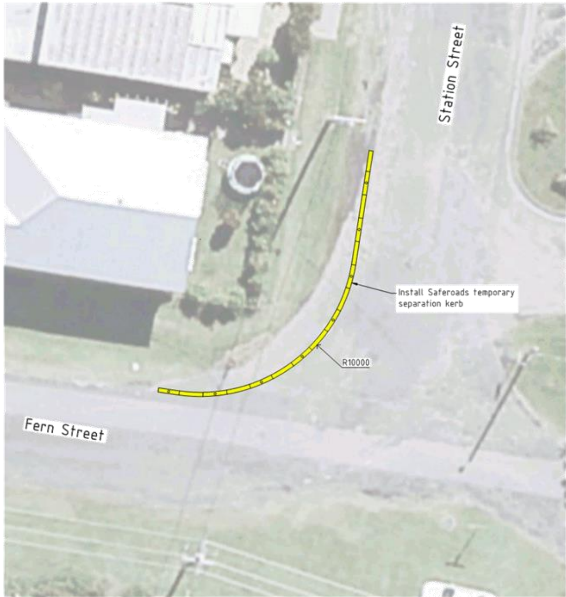
Site Plan - Fern St / Station St Intersection Scale 1:100 (A3)
