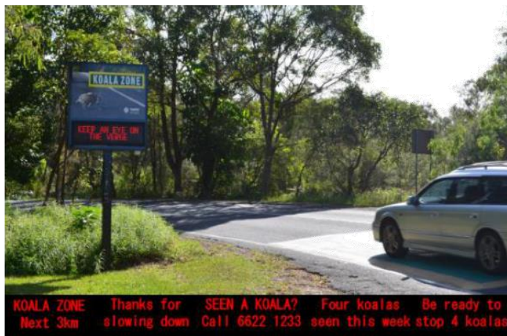
Plate 6. A constantly scrolling Variable Message Sign (VMS; not vehicle activated) manufactured by HIVIS Group and installed on Clothiers Creek Rd in the Tweed LGA (Source: S. Hetherington).
