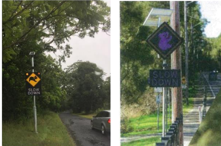
Plate 5. Koala Vehicle-Activated Signs (VAS) manufactured by Pioneerz Safety and installed on Bagotville Road in the Ballina LGA (left). Another version of koala VAS manufactured by HIVIS Group installed at Hawksnest on the mid-north coast (right). Signs are set to activate on a set speed (e.g. 5 km/h below the signed speed limit).
