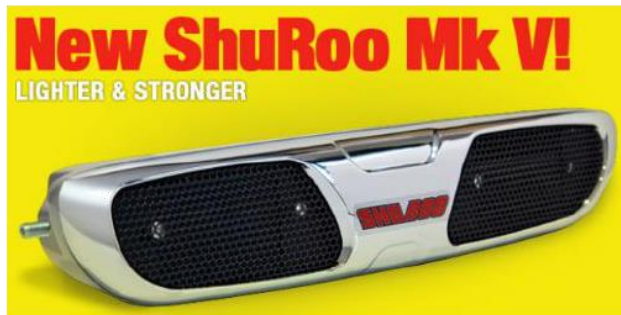
Figure 6. Audio deterrents such as the ShuRoo mount to the front of a vehicle and emit a pattern of high-frequency sounds intended to alert kangaroos and other wildlife of an approaching vehicle (Source: www.shuroo.com.au ).
