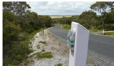
Figure 4. Virtual Fencing is distributed in Australia by Wildlife Safety Solutions. Approaching car headlights activate the sensor which emits sound and light to deter animals from crossing the road. (Source: www.wildlifesafetysolutions.com.au )
