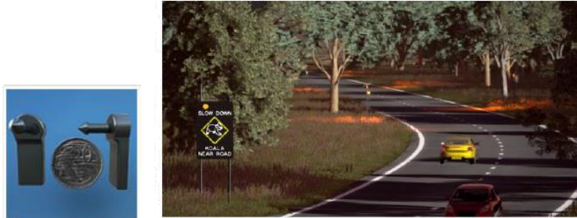
Figure 2. WID ear tag (left) and schematic of WID-activated signage system (right). (Source: www.wildspy.com.au ).
