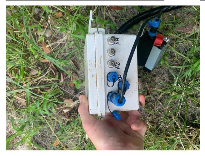
Figure 3: Tallow Creek water quality monitoring equipment at the Footbridge, after being vandalised (Photos taken 24 February 2021. Photo credit: T. Barchard).
