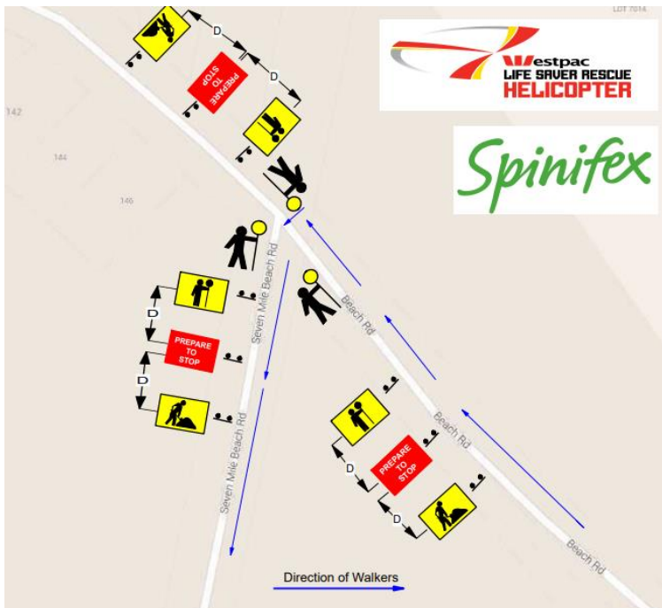
Figure 3 – Proposed TGS for the Seven Mile Beach Road entrance (refer Figure 2). The Traffic Control is to be in place from 6.30am to 2.30pm.
