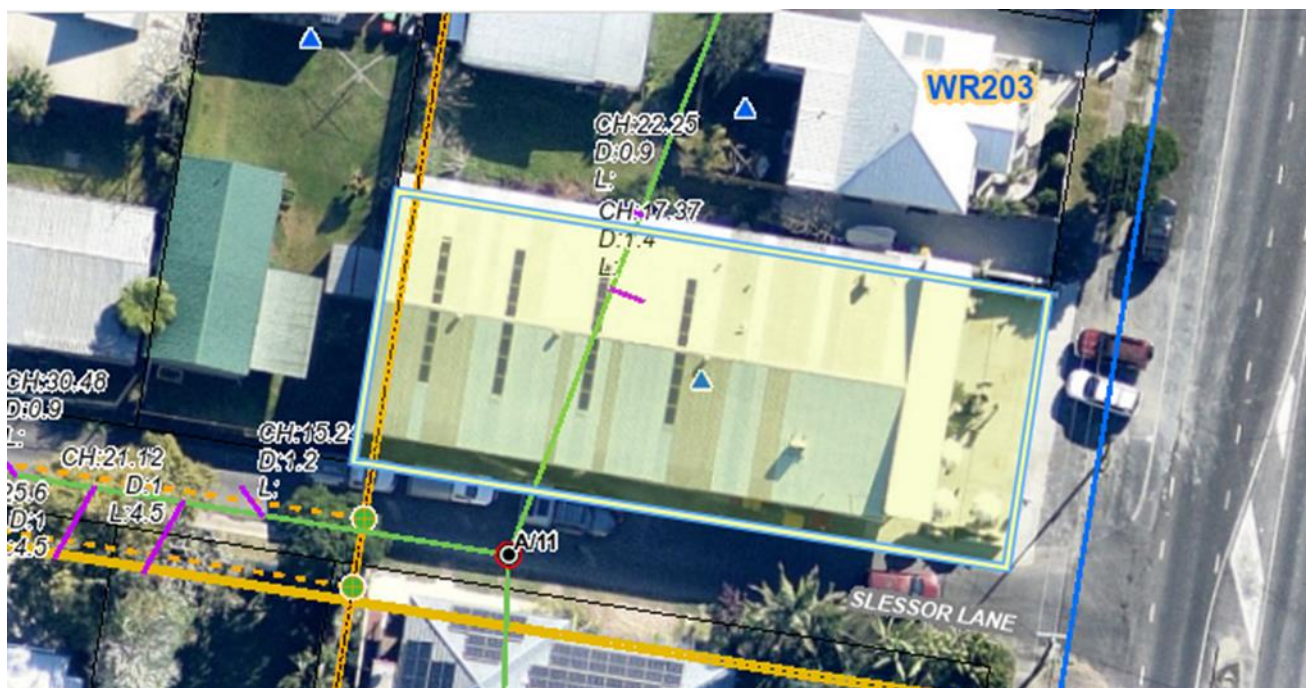
Figure 4: Infrastructure on site: stormwater (orange) sewer (green)
