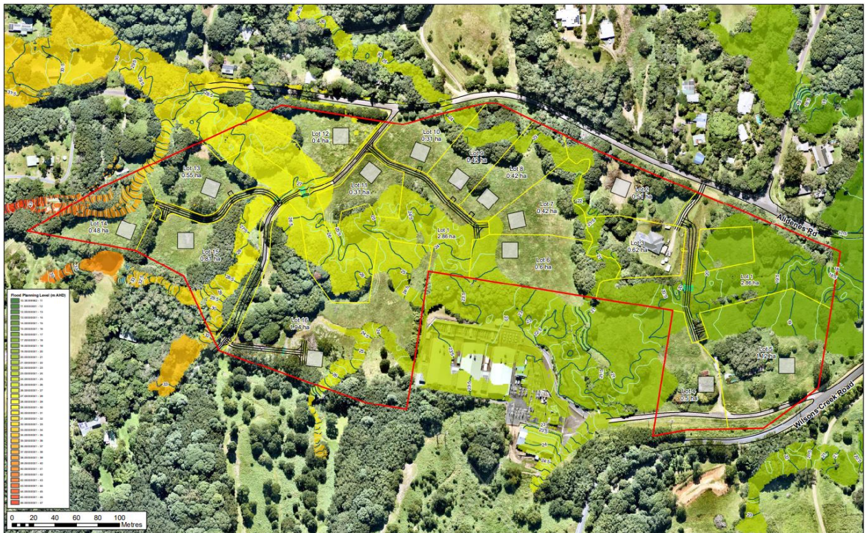
Figure 11: Extract of flooding map illustrating the extent of flooding during a 1% annual exceedance probability event. Proposed building envelopes are located on flood free land.
