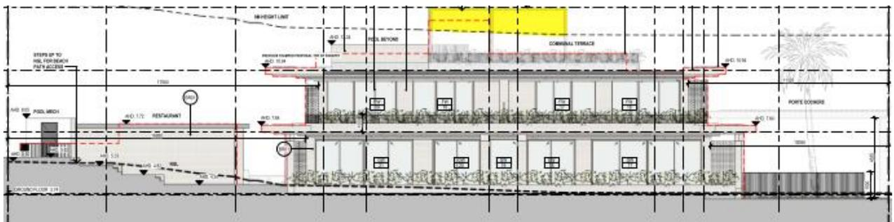
**Figure 18:** Extract of western elevation with 9m building height exceedance highlighted in yellow.
