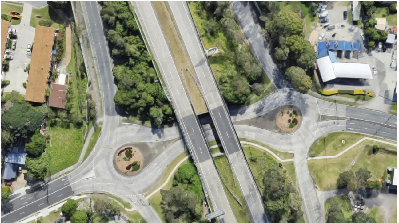
10 Figure 4. Example Dog-Bone Intersection Form (Kennedy Drive, Tweed Heads)
