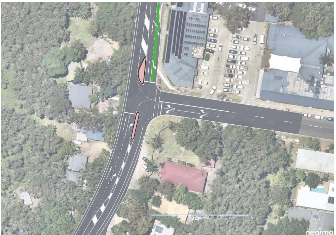
Figure 2. Option 1 – Traffic light intersection Concept Design
