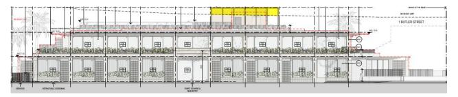
Figure 17: Extract of Shirley Street elevation with 9m building height exceedance highlighted in yellow.
