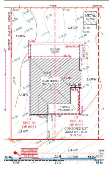
Figure 3: Extract of site plan showing footprint of existing dwelling and setbacks to the boundaries
