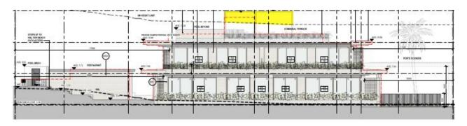
**Figure 18:** Extract of western elevation with 9m building height exceedance highlighted in vellow.
