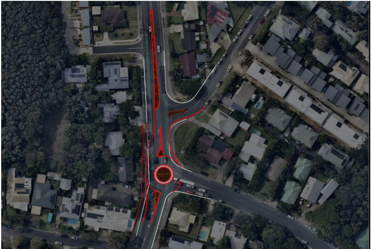
Figure 3. Indicative sketch of roundabout option
