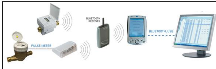
Figure 2: Typical Drive-by System Architecture
