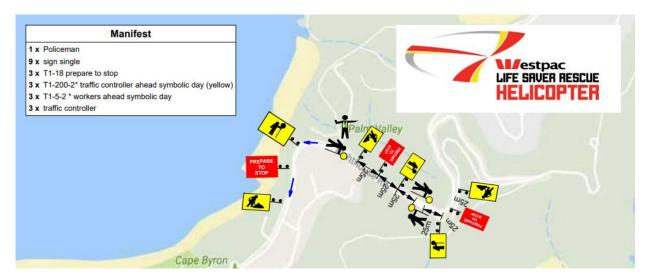
Figure 4 – Traffic control proposed for eastern section Lighthouse Road. Coming down from Lighthouse Road (refer to Figure 1). Traffic control to be in place from 6am to 10.30pm.
