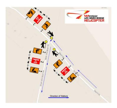
Figure 3 – Proposed TGS for the Seven Mile Beach Road entrance (refer Figure 2). The Traffic Control is to be in place from 7am to 1pm.
