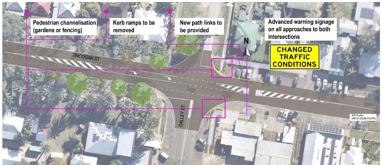
Figure 7: Associated works (Tincogan St/Dalley St intersection)
