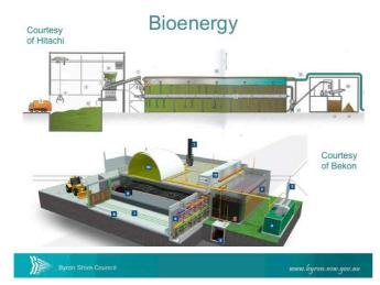
however, the HZI PFR comes with a higher CAPEX and also generates considerable volume of liquid digestate that must also be managed. The Bekon batch tunnel process is less costly to build and less complex technologically, but also has a greater need for mobile plant and manual labour requirements. Furthermore, the HZI and Bekon solid digestates are not of the same quality or quantity, and require different handling prior to reuse.
