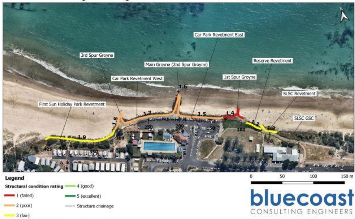
Figure 3: Structural condition rating for structure based on visual and drone inspection on 28 th October 2019.
