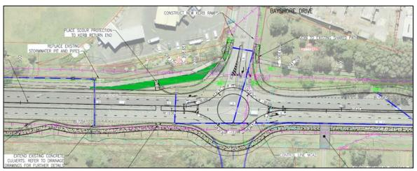
The merge lane length for the upgraded roundabout on Ewingsdale Road with the access to the sports fields indicates a lane and merge length of 202m. To determine the appropriate length to transition from two circulating lanes to one lane reference is made to Austroads Guide to Rod Design Part 4B: Roundabouts Clause 4.3.4.
