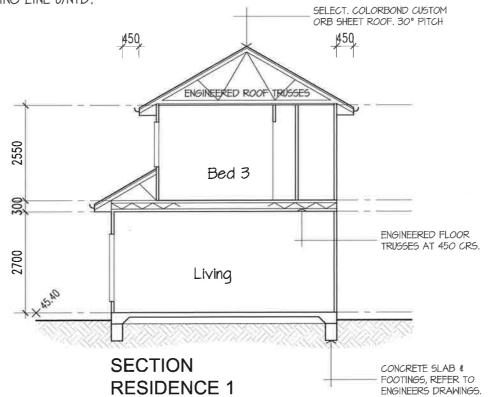
NOTE - FOR ALL STRUCTURAL, BRACING & TIE DOWN DETAILS, REFER TO ENGINEERS DRAWINGS
