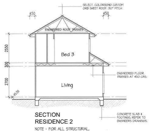
NOTE - FOR ALL STRUCTURAL, BRACING & TIE DOWN DETAILS, REFER TO ENGINEERS DRAWINGS
