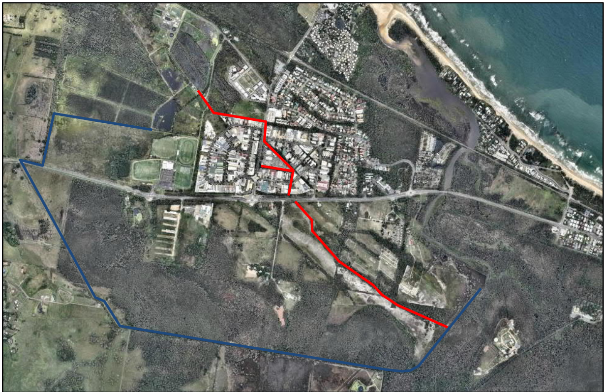
Figure 1. Historical (blue) and new (red) Byron Bay STP excess effluent discharge pathways
