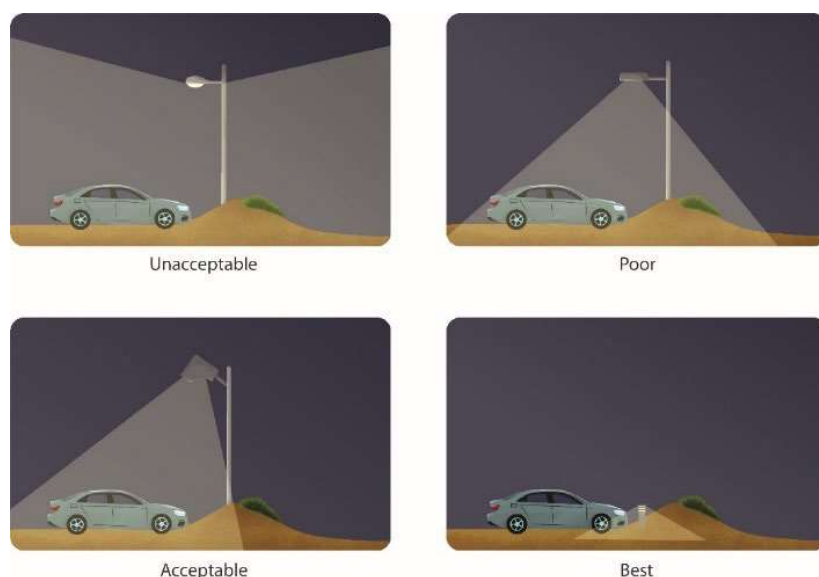
Figure 14 Lighting options for a parking area
