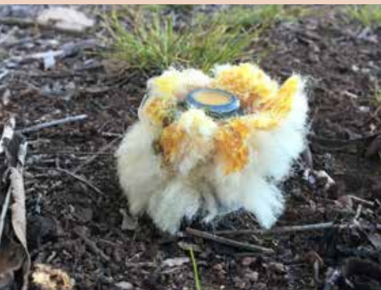
An active CPE with lamb's wool-lure coated in fish oil. Source: Lana Harriott, Biosecurity Queensland, Department of Agriculture and Fisheries.
