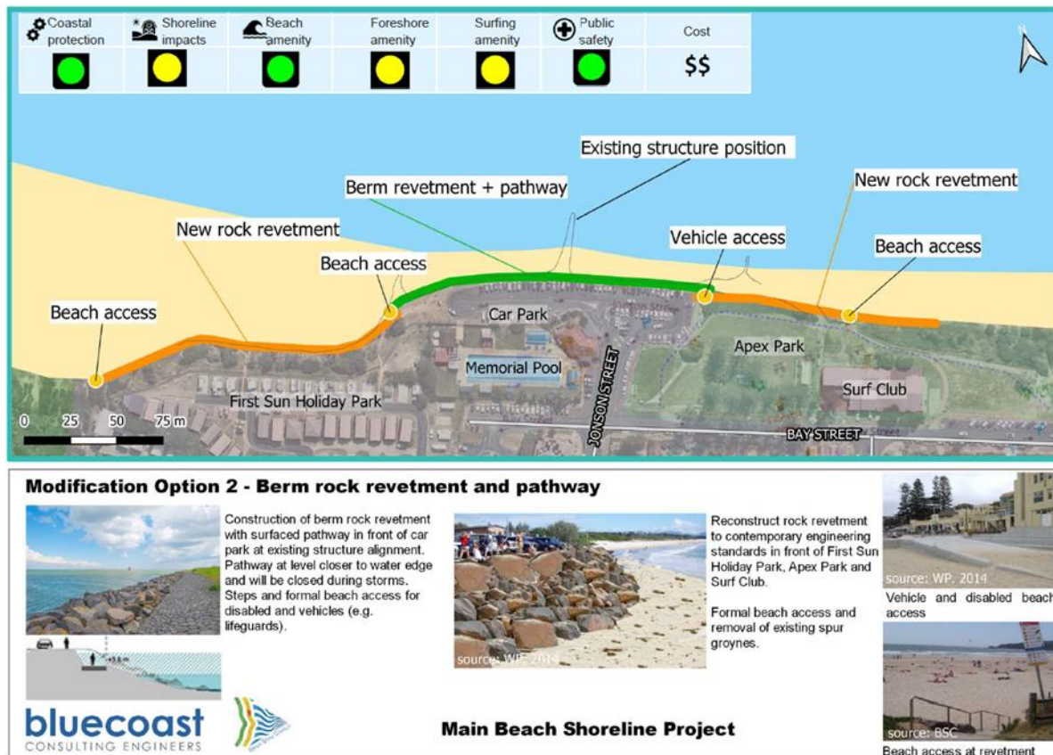
Figure 5: Modification option 2 – berm rock revetment.
