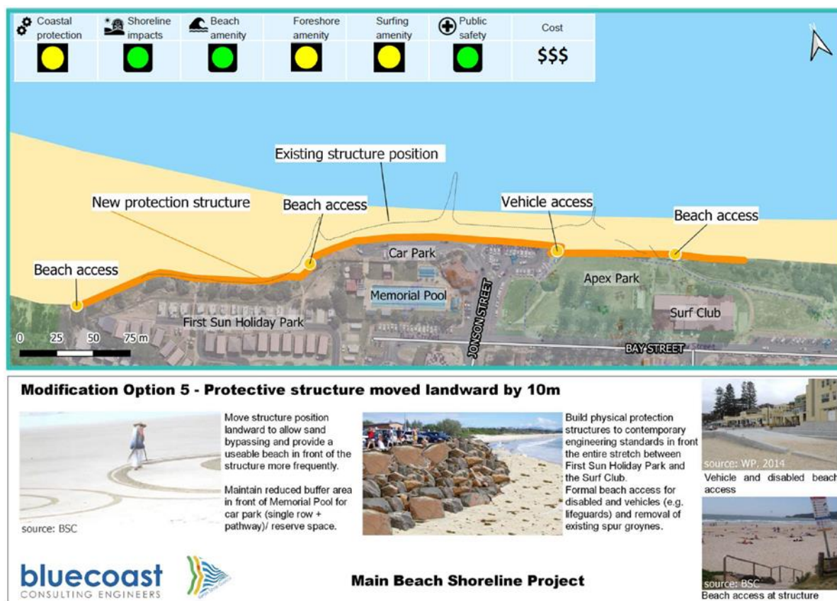
Figure 9: Option 5 – protective structures moved landward by 10m.
