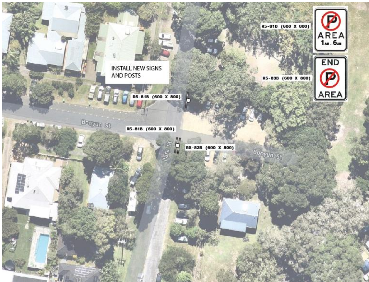
Figure 1: Signage installation Plan
