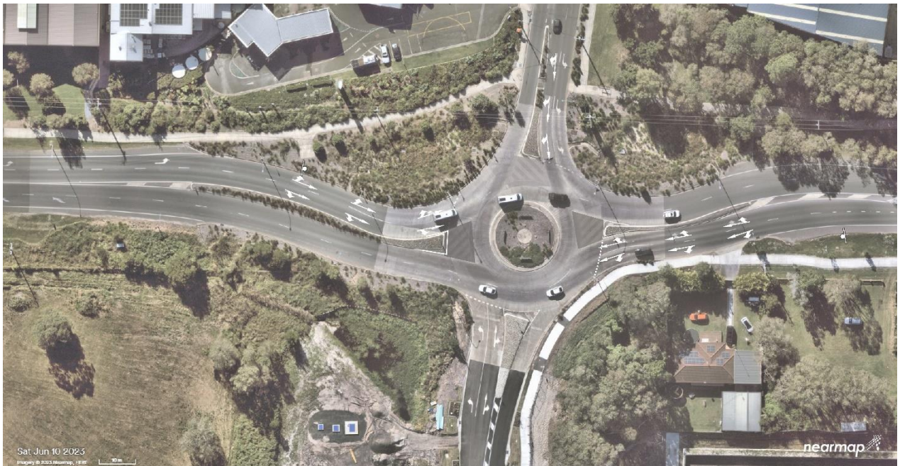
Figure 5: No circulating delineation within the east and west sections of the circulating lane
