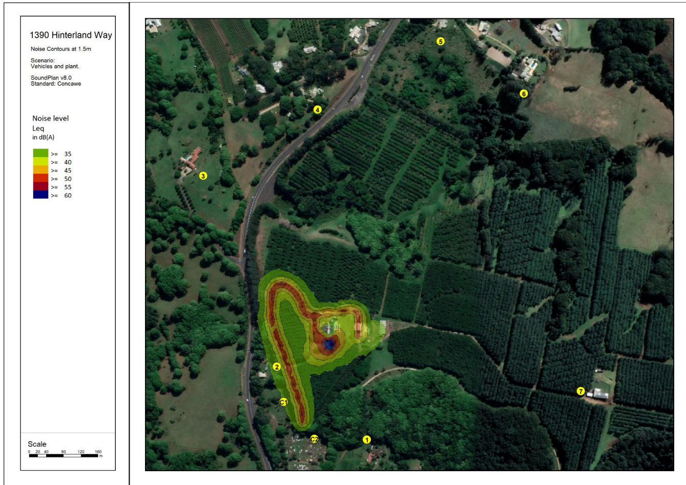
Plate 3.4 Noise contours at 1.5m above ground, standard meteorology, vehicle movements, cool room, generator and catering noise sources operating. Levels are in dB(A) Leq
