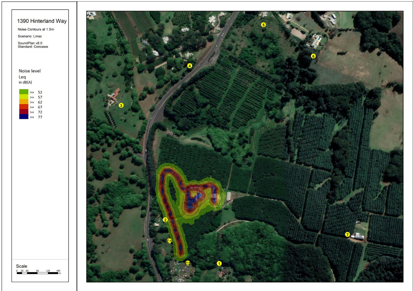
Plate 3.8 Noise contours at 1.5m above ground, standard meteorology, Vehicle movements, car door closures and patrons at all event areas (Lmax, night). Levels are in dB(A) Lmax.
