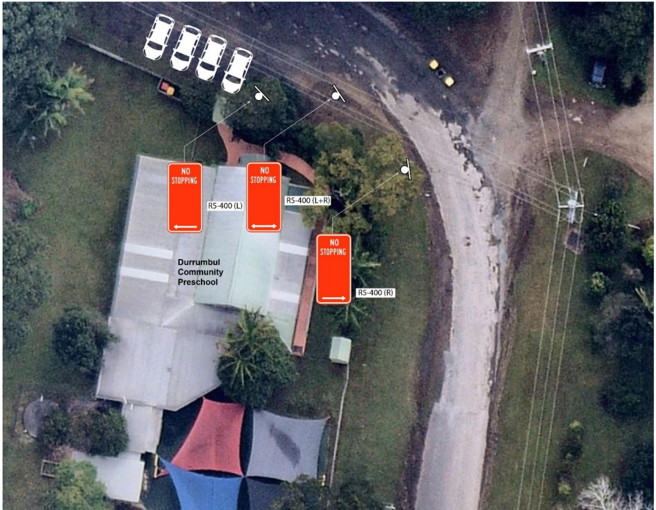
Figure 3: Propose Sign Installation (above)
