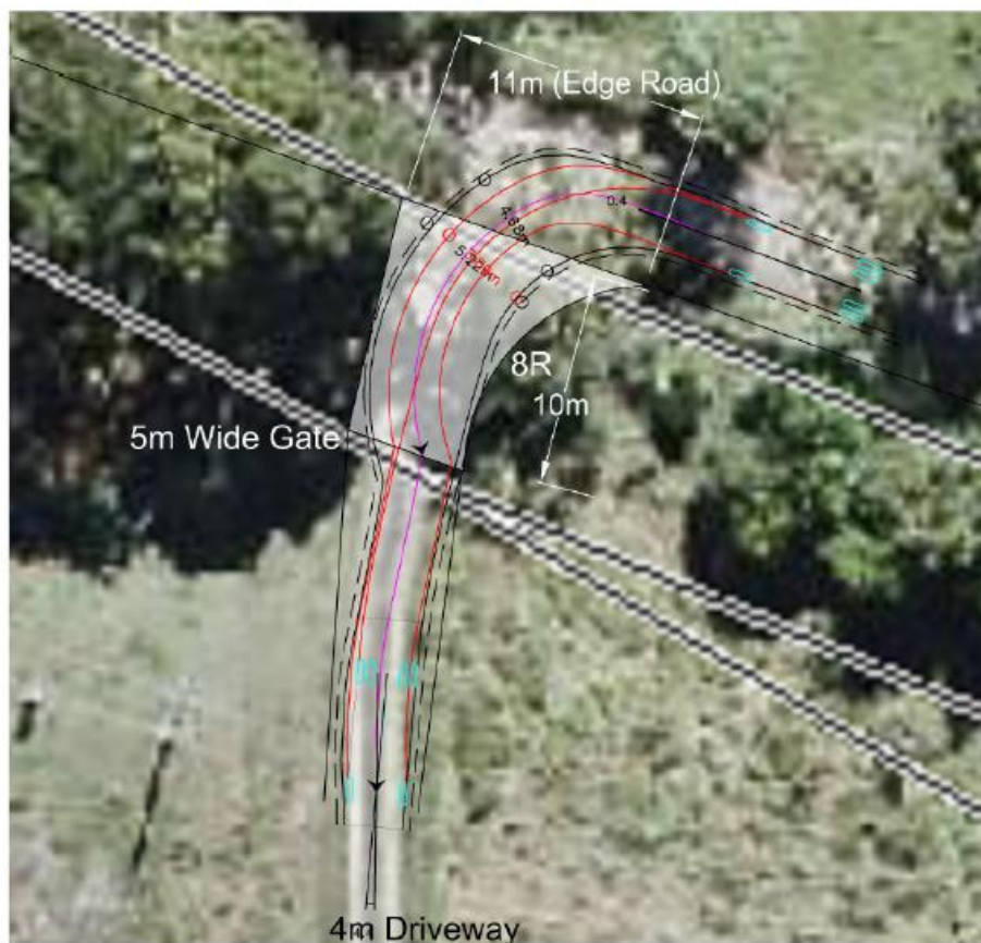
Figure 3.3 Turning Template Assessment of Works Required
