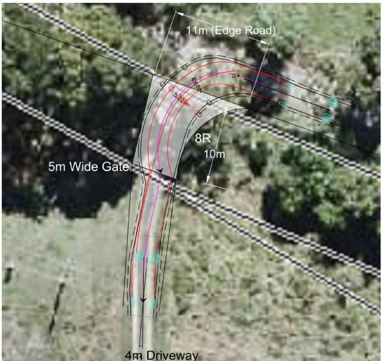
Figure 3.3 Turning Template Assessment of Works Required
