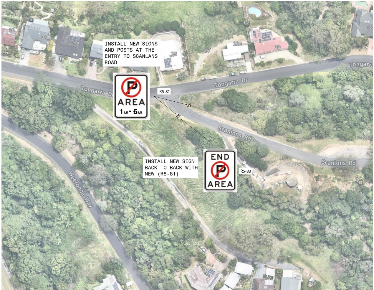
Figure 1: Devine Hill no parking signage plan
