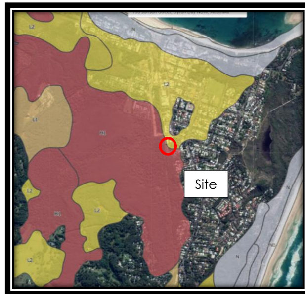
Diagram 2: Acid Sulfate Soil Risk Map for Site
