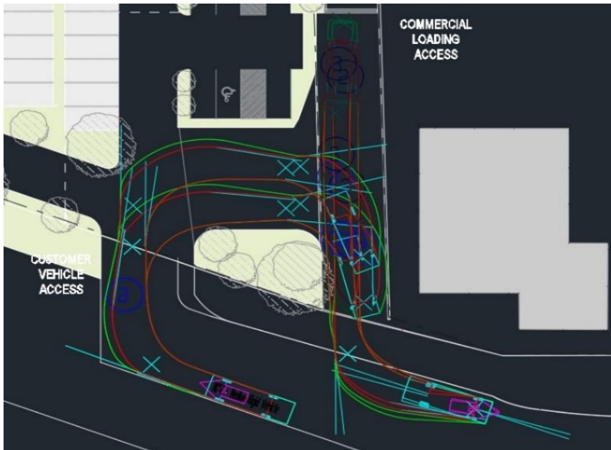
Figure 4 | 2 x MRV turning movements into Loading Bay
