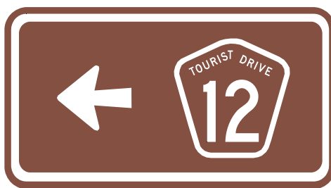
Figure 3.45 Example of ADVANCE GUIDANCE MARKER (G8-203)
