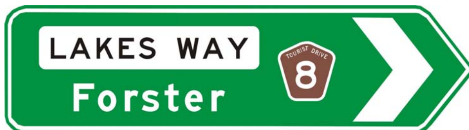
Figure 3.43 Example of INTERSECTION DIRECTION (G2-1) sign incorporating regional tourist drive route marker
