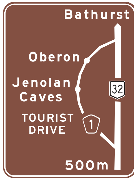
Figure 3.40 Example of DIAGRAMMATIC ADVANCE DIRECTION (G8-208) sign
