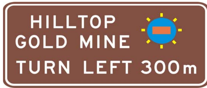
Figure 3.54 Example of ADVANCE (G11 series) sign with a themed touring route logo
