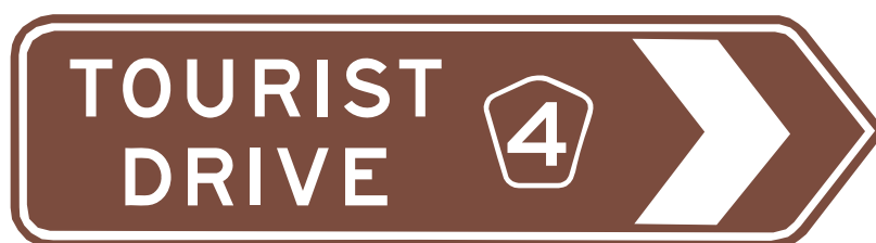
Figure 3.41 Example of INTERSECTION DIRECTION (G8-9-5) sign
