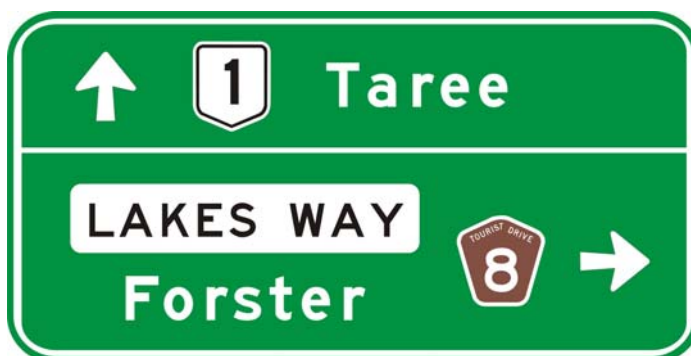
Figure 3.39 Example of ADVANCE DIRECTION (G1-202) sign incorporating regional tourist drive route marker
