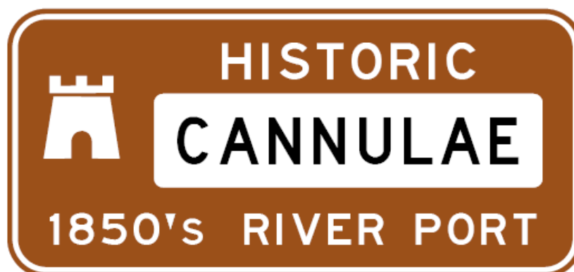
Figure 3.17 Example of TOWN NAME (G11-201) sign for an historic town or village
