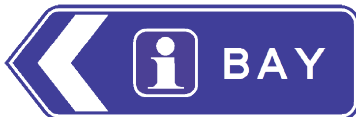
Figure 3.22 Example of an INFORMATION BAY or LAY-BY INTERSECTION (G7-4-1) sign
