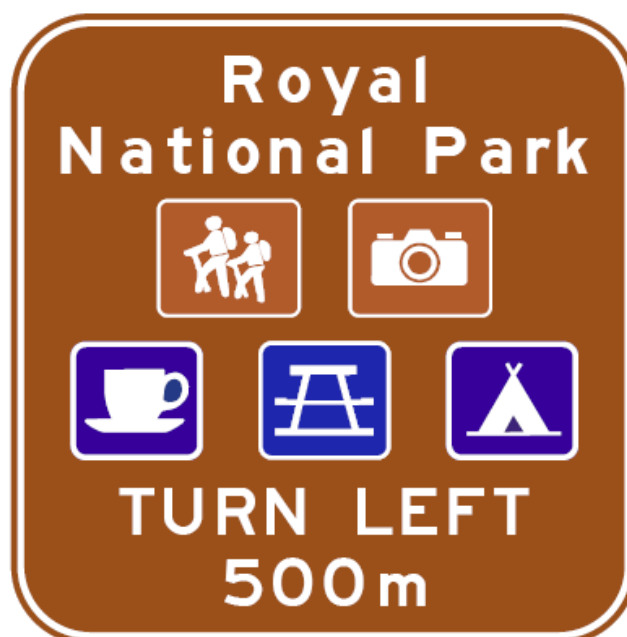
Figure 3.18 Example of an ADVANCE DIRECTION (G11-209) sign
