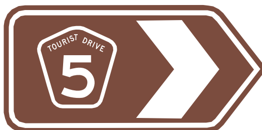
Figure 3.46 Example of INTERSECTION GUIDANCE MARKER (G8-204)
