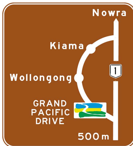
Figure 3.56 Example of DIAGRAMMATIC TOURING ROUTE ADVANCE DIRECTION (G11-217) sign
