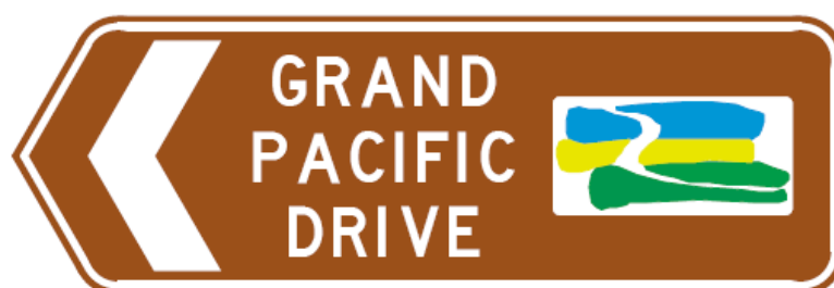
Figure 3.58 Example of TOURING ROUTE INTERSECTION DIRECTION (G11-219) sign
