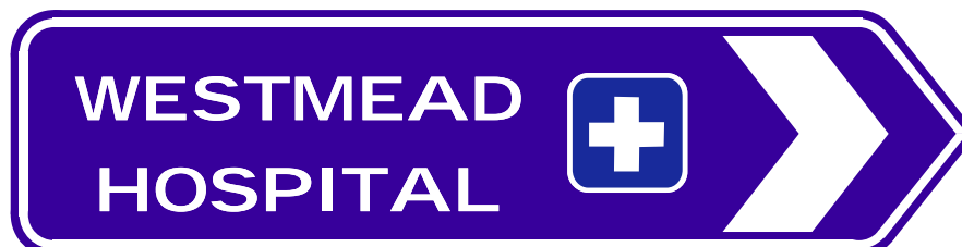
Figure 5.4 Example of INTERSECTION DIRECTION (G7 series) sign leading to a hospital, or, for use at the hospital entrance [G7-287 (top) and G7-288 (bottom)]
