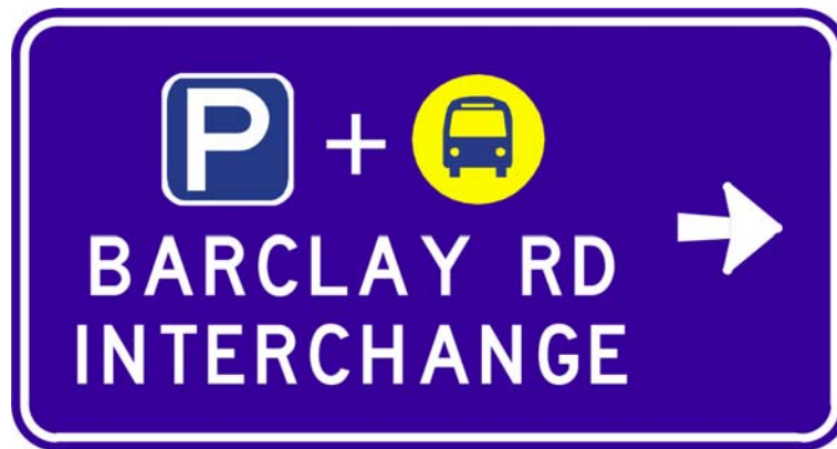
Figure 11.5 Example of an ADVANCE DIRECTION (G7-304) sign to a bus interchange car park
