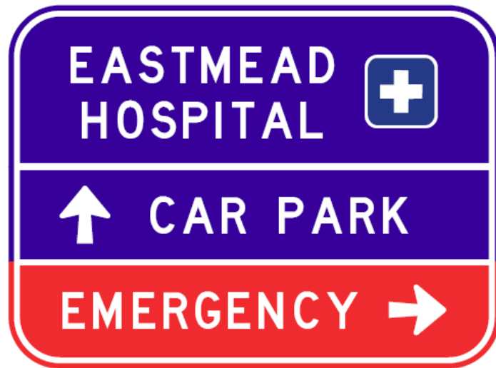
Figure 5.5 Example of HOSPITAL ADVANCE DIRECTION (G7-310) sign where the visitor car park and emergency services have separate access points
