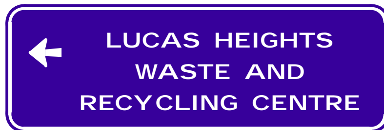
Figure 13.1 Example of an ADVANCE DIRECTION (G1 series) sign to a waste and recycling centre
