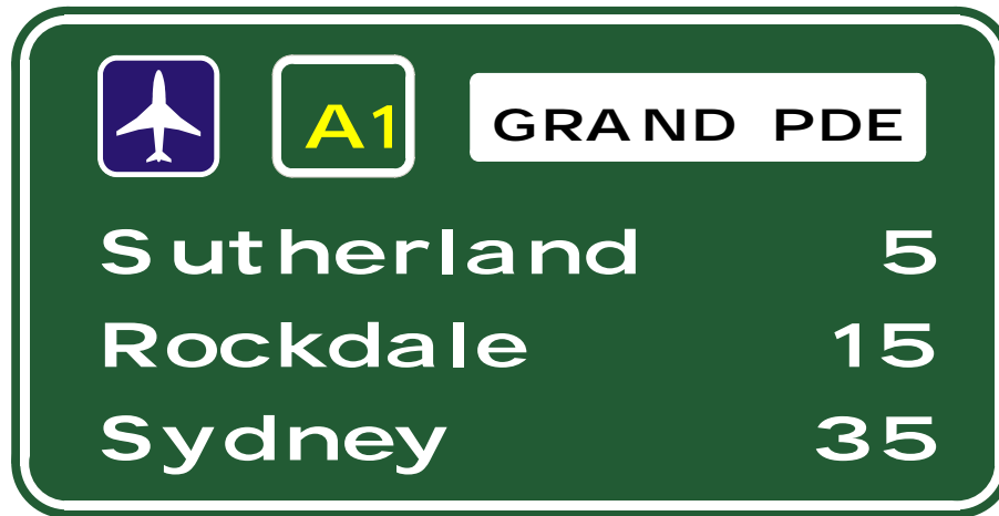
Figure 6.7 Example of broader cordon AIRPORT REASSURANCE DIRECTION (G4-1) sign
