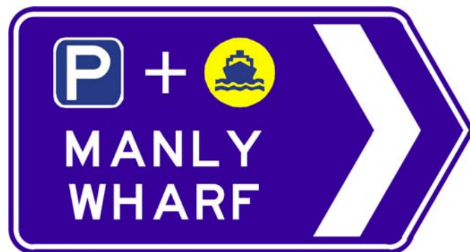
Figure 11.8 Example of an INTERSECTION DIRECTION (G7-305) sign to a ferry wharf car park
