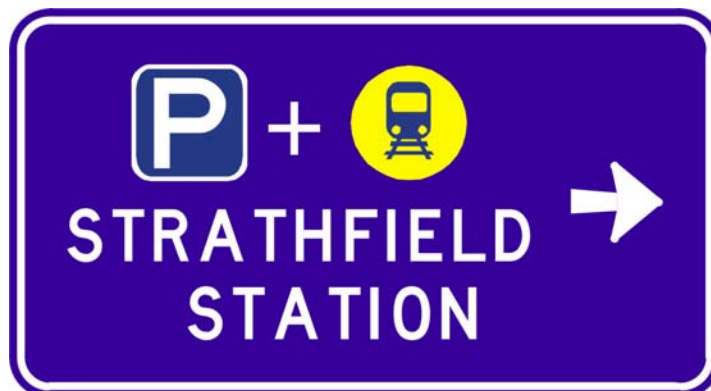
Figure 11.3 Example of an ADVANCE DIRECTION (G7-304) sign to a railway station car park
