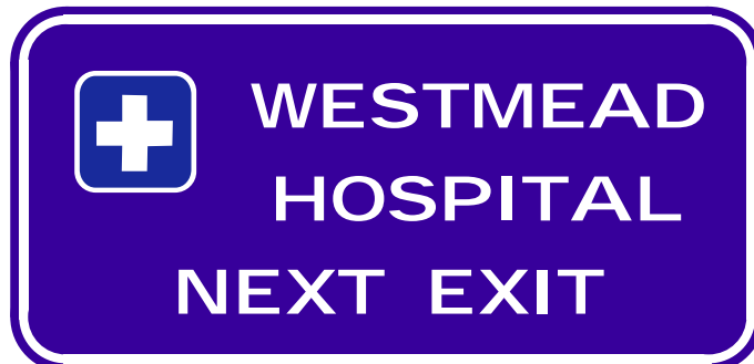
Figure 5.1 Example of HOSPITAL EXIT (GE7-216) sign
