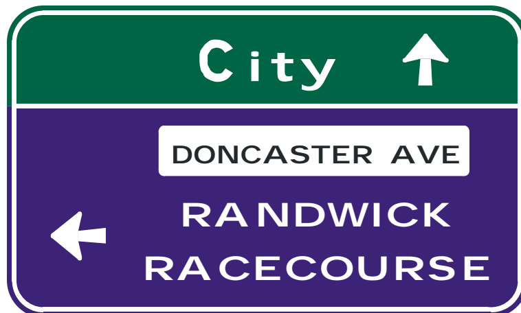
Figure 10.2 Example of an ADVANCE DIRECTION (G1-1) sign to a major sporting venues
