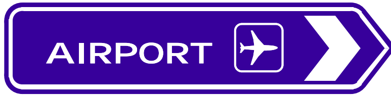
Figure 6.9 Example of regional AIRPORT INTERSECTION DIRECTION (G7-291) sign
