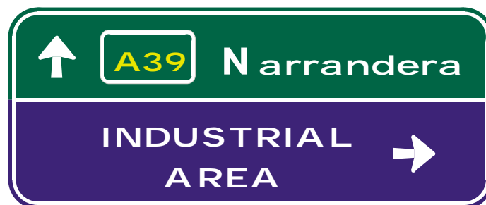
Figure 9.2 Example of ADVANCE DIRECTION (G1 series) sign to an INDUSTRIAL AREA or BUSINESS PARK
