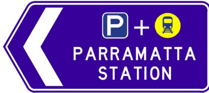
Figure 11.4 Example of an INTERSECTION DIRECTION (G7-305) sign to a railway station car park
