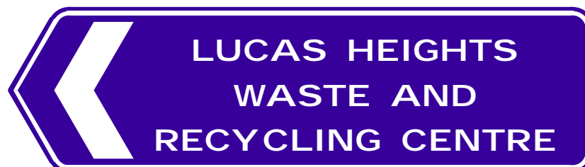
Figure 13.2 Example of an INTERSECTION DIRECTION (G2-1) sign to a waste and recycling centre
