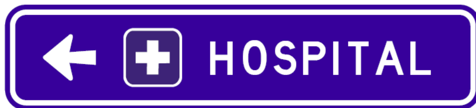
Figure 5.2 ADVANCE DIRECTION (G7-307) sign for a hospital, where no town name is required
