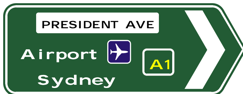
Figure 6.3 Example of inner cordon AIRPORT INTERSECTION DIRECTION (G2-I) sign
