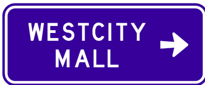
Figure 8.1 Example of REGIONAL SHOPPING CENTRE ADVANCE DIRECTION (G7-297) sign
