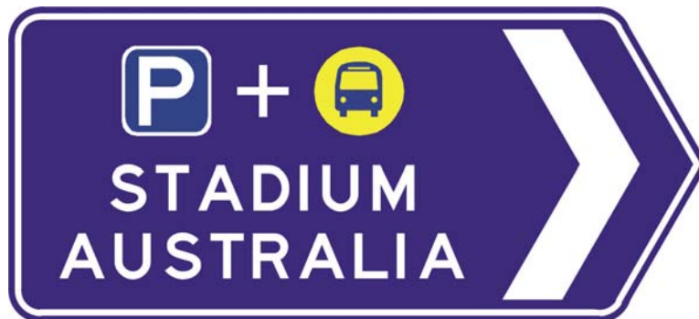
Figure 11.2 Example of an INTERSECTION DIRECTION (G7-305) sign to a park and ride facility car park
