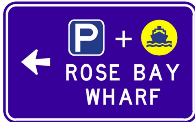
Figure 11.7 Example of an ADVANCE DIRECTION (G7-304) sign to a ferry wharf car park
